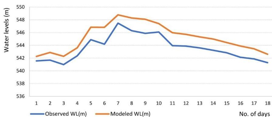
Fig. 6. Calibrated water level profiles (stages) at Phulgaon gauging station (from 20 July 2005 to 8 August 2005).
